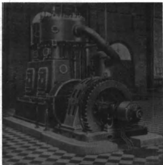
9. A two-stage air compressor made by Tilghmans (1911). (From company brochure, pre-1914.)
